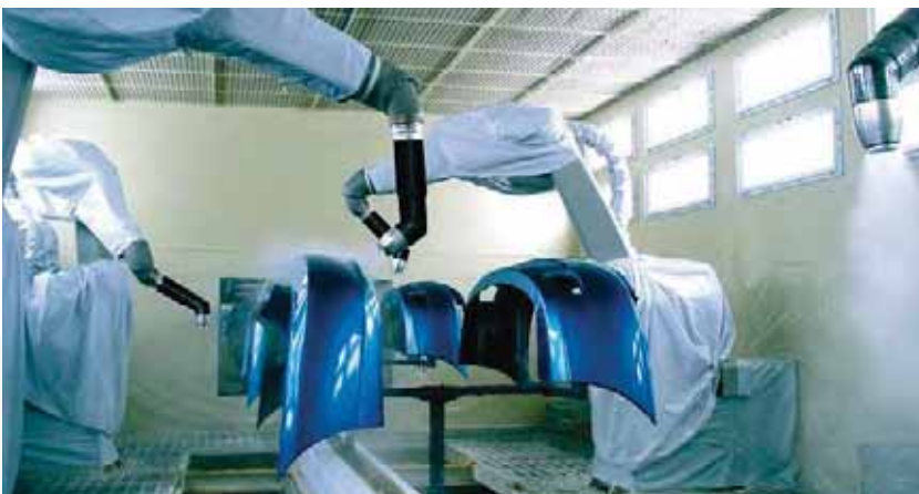
Clear coat application on bumper - PPH 707 SB
