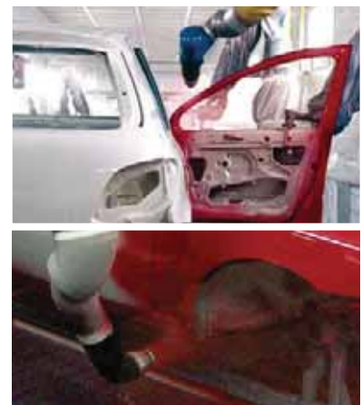
Base coat 1 cut-in - ACCUBELL 608 or PPH 707 SB
